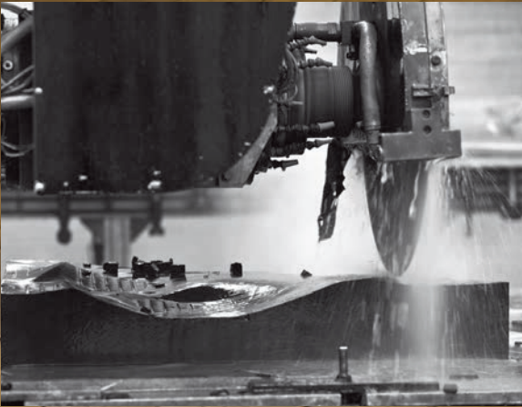
2 Rotating saws slowly cut the marble lengthways, moving up and down in keeping with the CGI-designed template. The saw worked on the marble without pause for two weeks, cutting lines 5mm thick.
